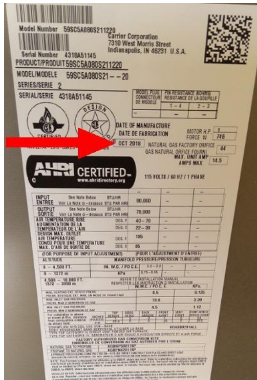
Photo of the manufacturer label. Arrow to indicate the manufacturer date. Oct. 2018
